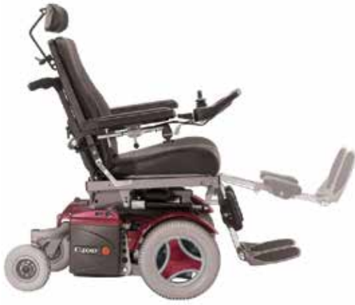
Figure 11: Power chair with elevating leg rests
