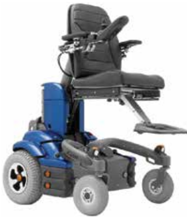
Figure 12: Power chair with a seat elevator
